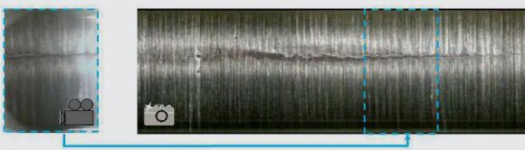
Reconstruction of an indication with the Stitching image processing tools: suppresion of distortions, ROI application and contrast enhancement
